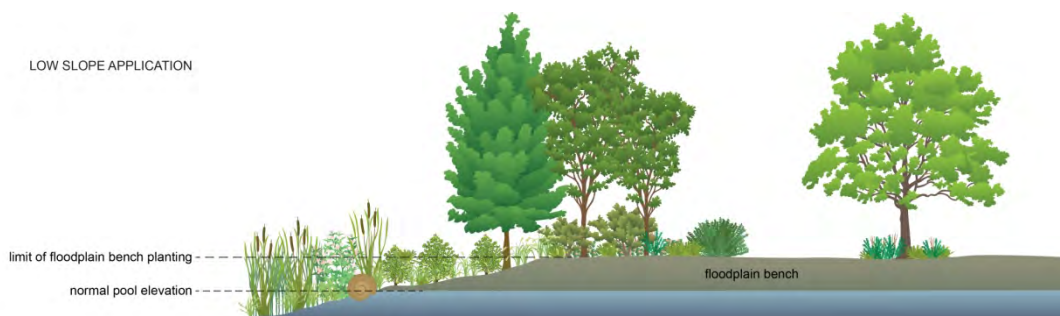
Figure 3.2. Floodplain bench restoration approach (Source: Biohabitats; August 4, 2015).
